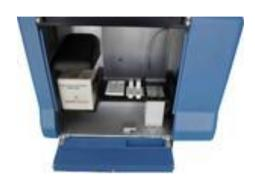
**RAFFAELLO** uses supported cellulose acetate strips which are managed completely automatically. Simply insert them in the appropriate slots and tell the machine which strips to use.
